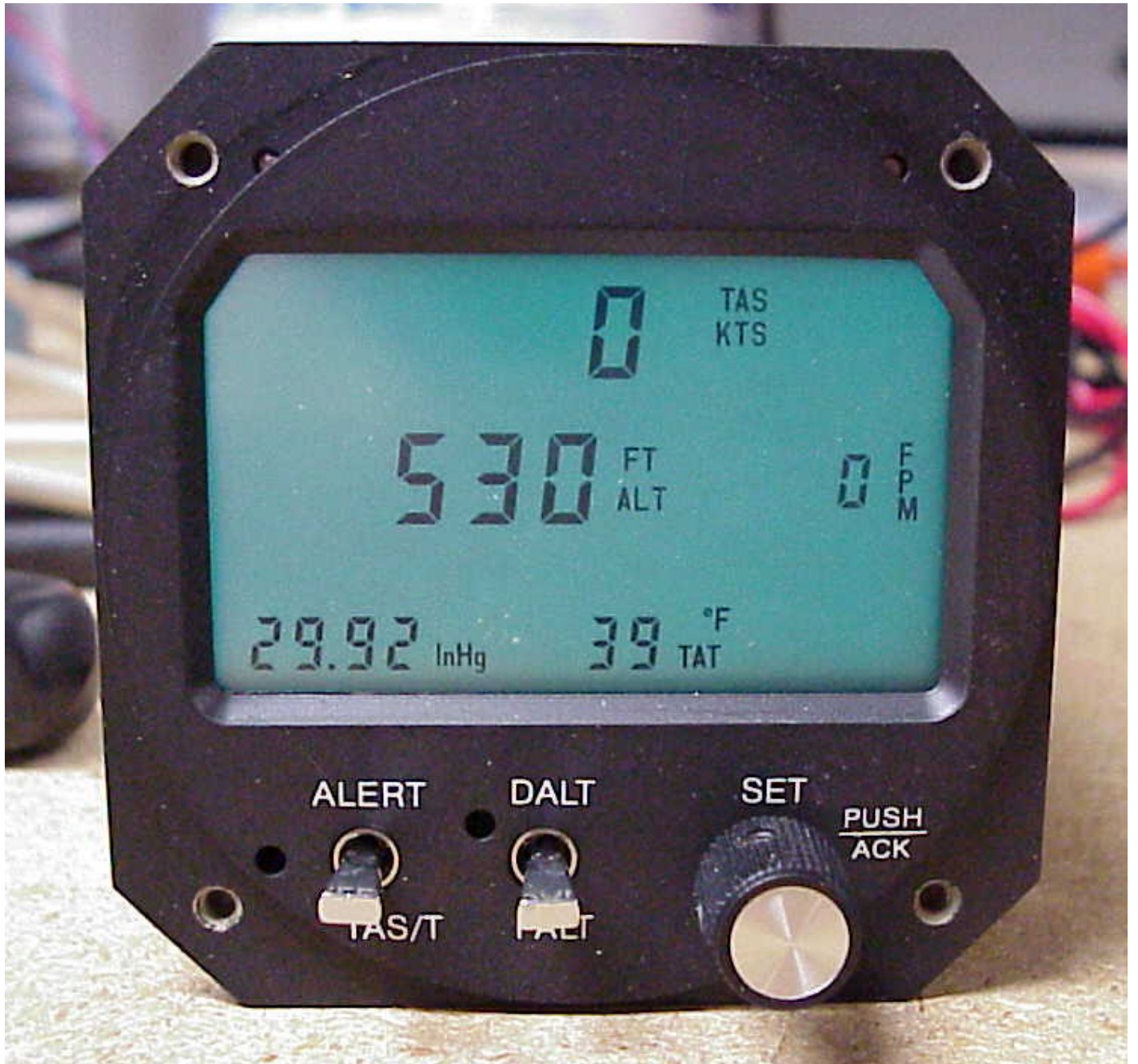
Rocky Mountain Instrument's popular microEncoder. It can be used as your airspeed indicator, altimeter, VSI, OAT gauge, and transponder encoder. See "Birth of a Panel" inside for the story.
