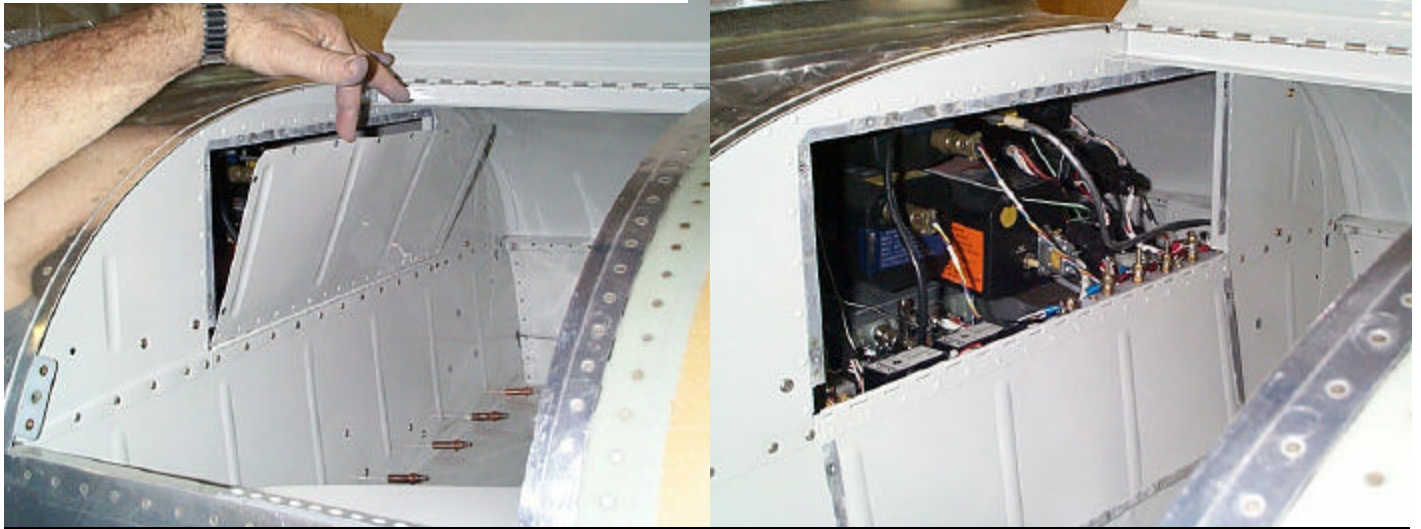
Access panels in the F-8XX bulkhead are a popular mod for RV-8 builders. These pictures from RV-8 builder Danny Lee of North Carolina, posted to the RV-8 OneList, depict an especially useful design.
