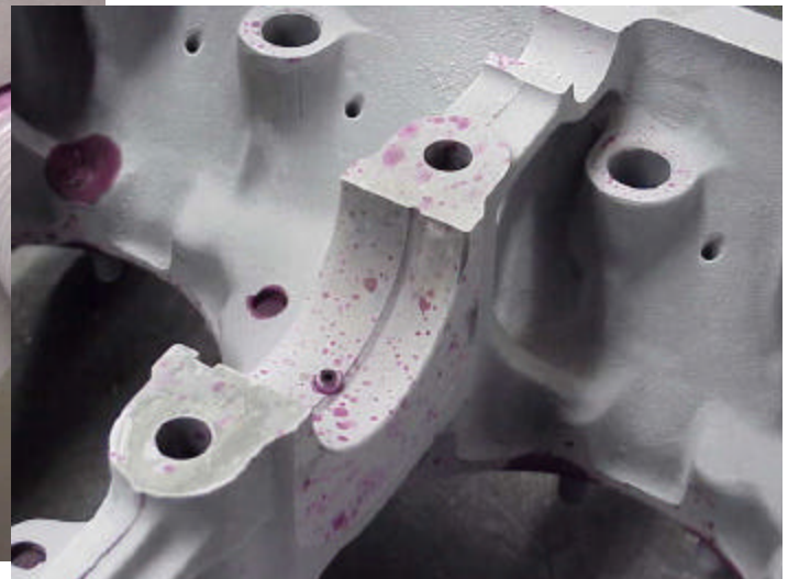
Top left; our host welcomes us to where it all starts. Top right; jugs everywhere! Bottom left; a crank after going through the dye penetrant process for crack inspection. Those purple marks are cracks that will each be fixed in the next step of the process. Bottom right; a crank bearing journal after the same process. The purple marks on the bearing face are metal fretting, probably from an improperly torqued bolt.
