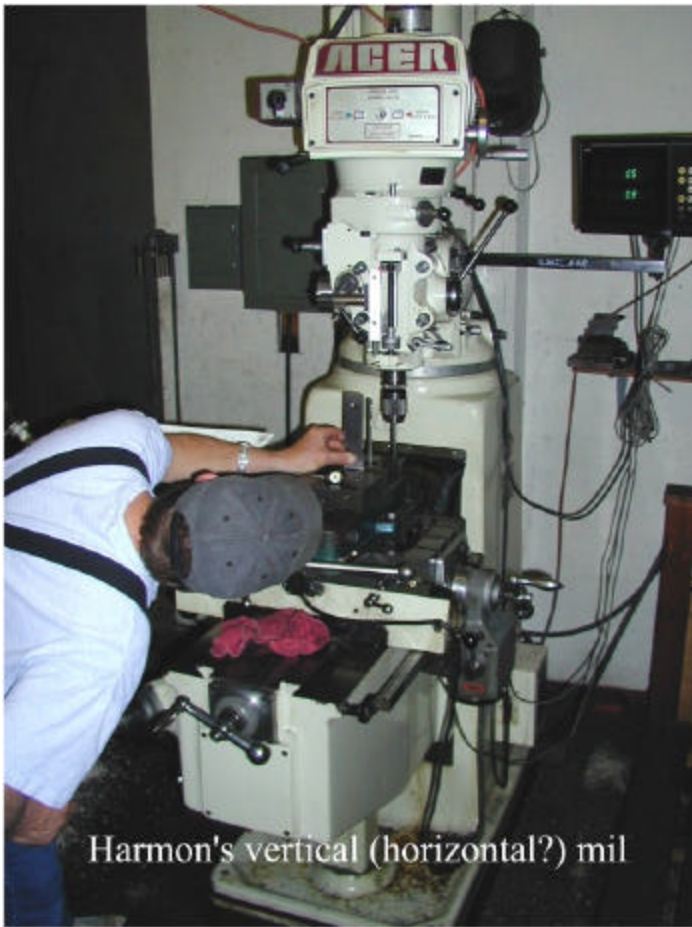
swivel dial indicator finds true center when rotated in chuck
