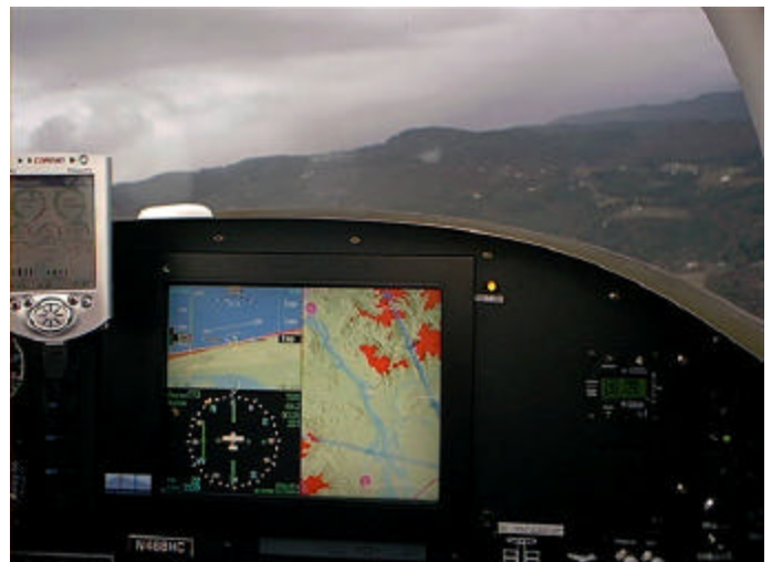
Harmon's new Blue Mtn. EFIS and IPAQ based engine monitor keep him informed!
