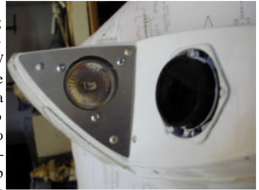
Landing/taxi light mounts inside wingtip lens (nav light is Home Depot under cabinet light)
