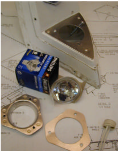
Typical "keep it simple" approach to a landing/taxi light system
