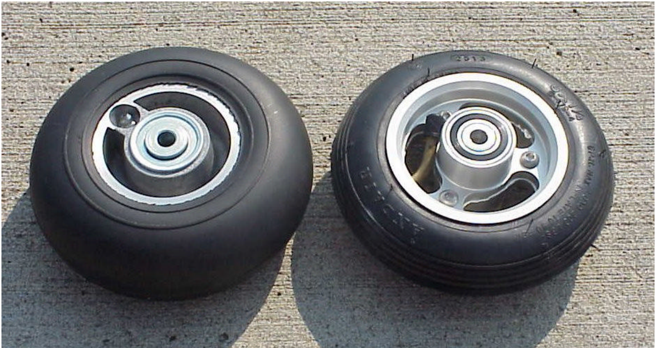
New Andair lightweight pneumatic tailwheel next to Van's hard rubber unit.
